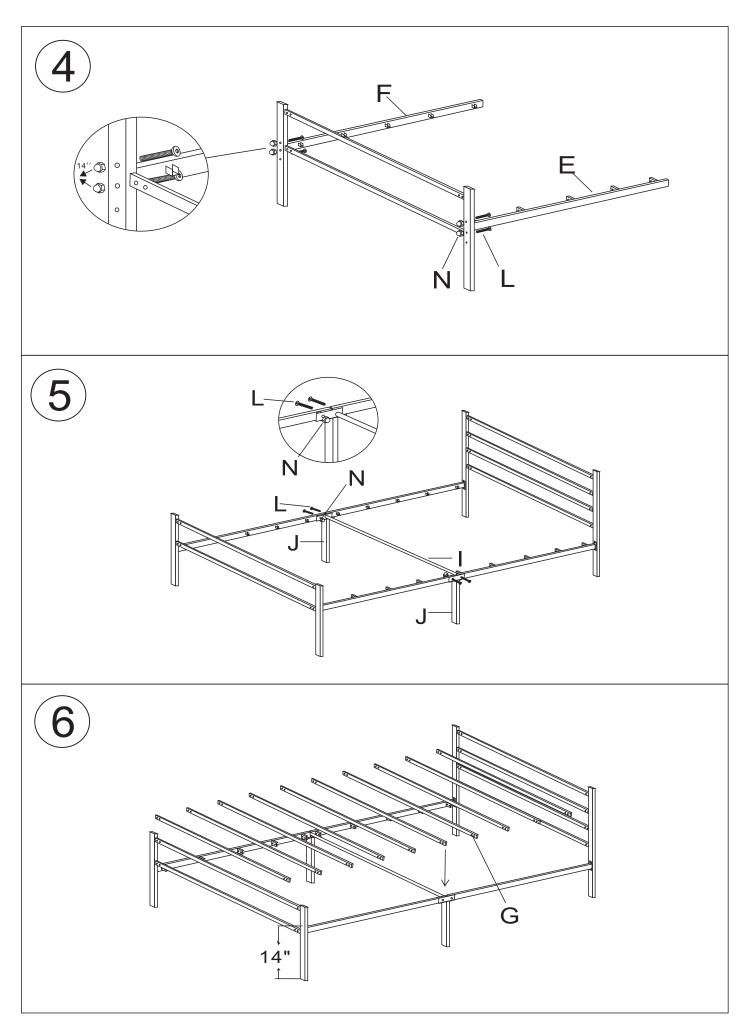
Note:During the installation process,the screws should not be tightened too tightly,After all the parts are installed,adjust them on a flat ground, and finally tighten the screws
